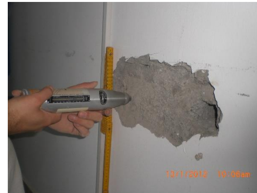
Concrete strength measuring (Schmidt hammer)
